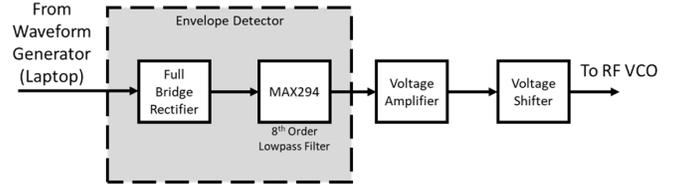
Fig. 3. Waveform Generation Stage Design.
