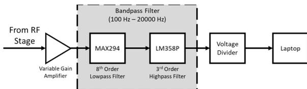
Fig. 2. Receive Audio Stage Design
