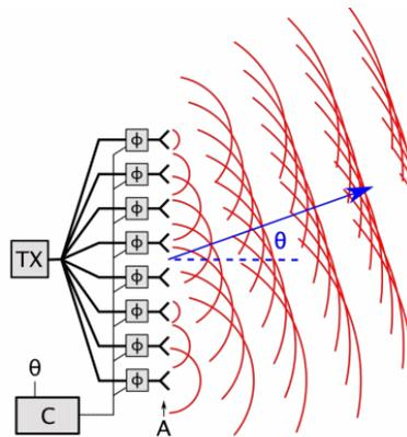
Figure 1: A schematic showing a phased array steering the signal
