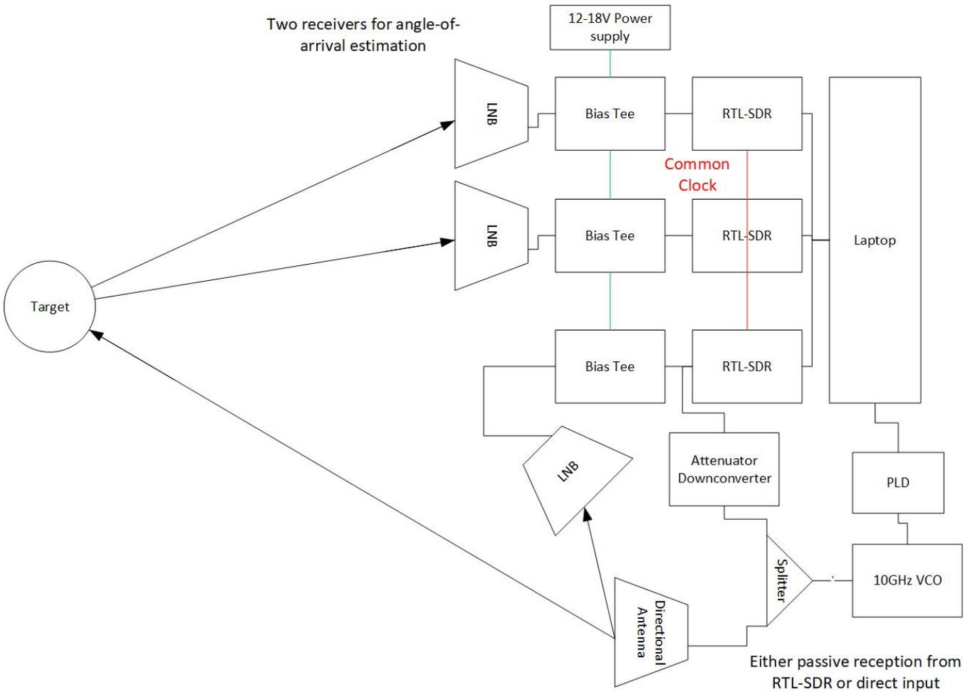
Figure 1: Super Cheap, X-Band, SDR Radar
