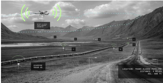
Combination of airborne cameras and ground-based radars (Echodyne Echoguard) https://dronebelow.com/2019/08/02/first-ever-bvlos-drone-operation-without-visual-observers/
