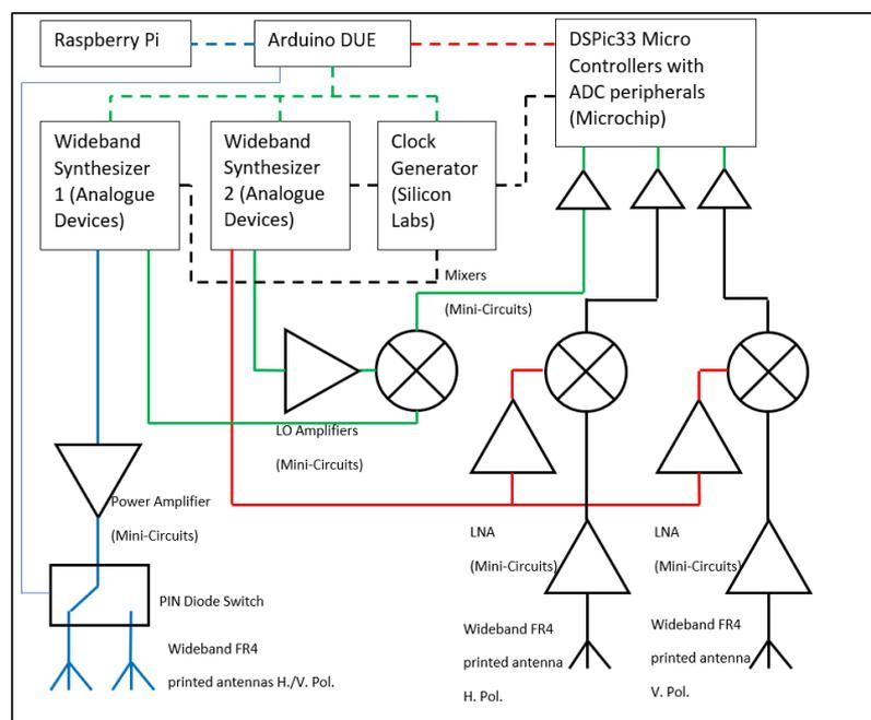
Figure 1 – System Block/Circuit Diagram
