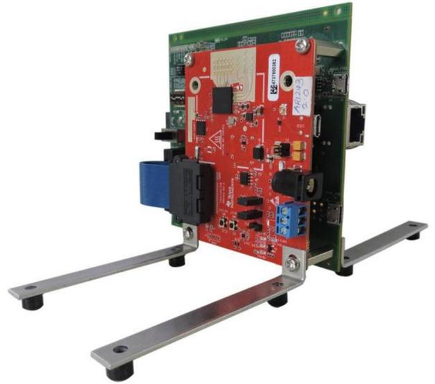
Figure 9: DCA1000EVM and IWR1843BOOST mounted with ribbon cable connection
